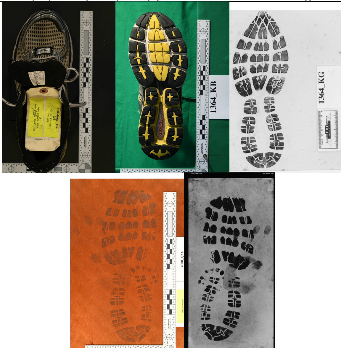
Fig S1. Source images for footwear item #1364, which was released as QK134 (shown in Fig S2). Note the use of preprinted labels in images. The image of the upper includes the specific substrate assigned to this shoe (H13S refers to this specific hardwood board). Only one of the five outsole images is shown here.
