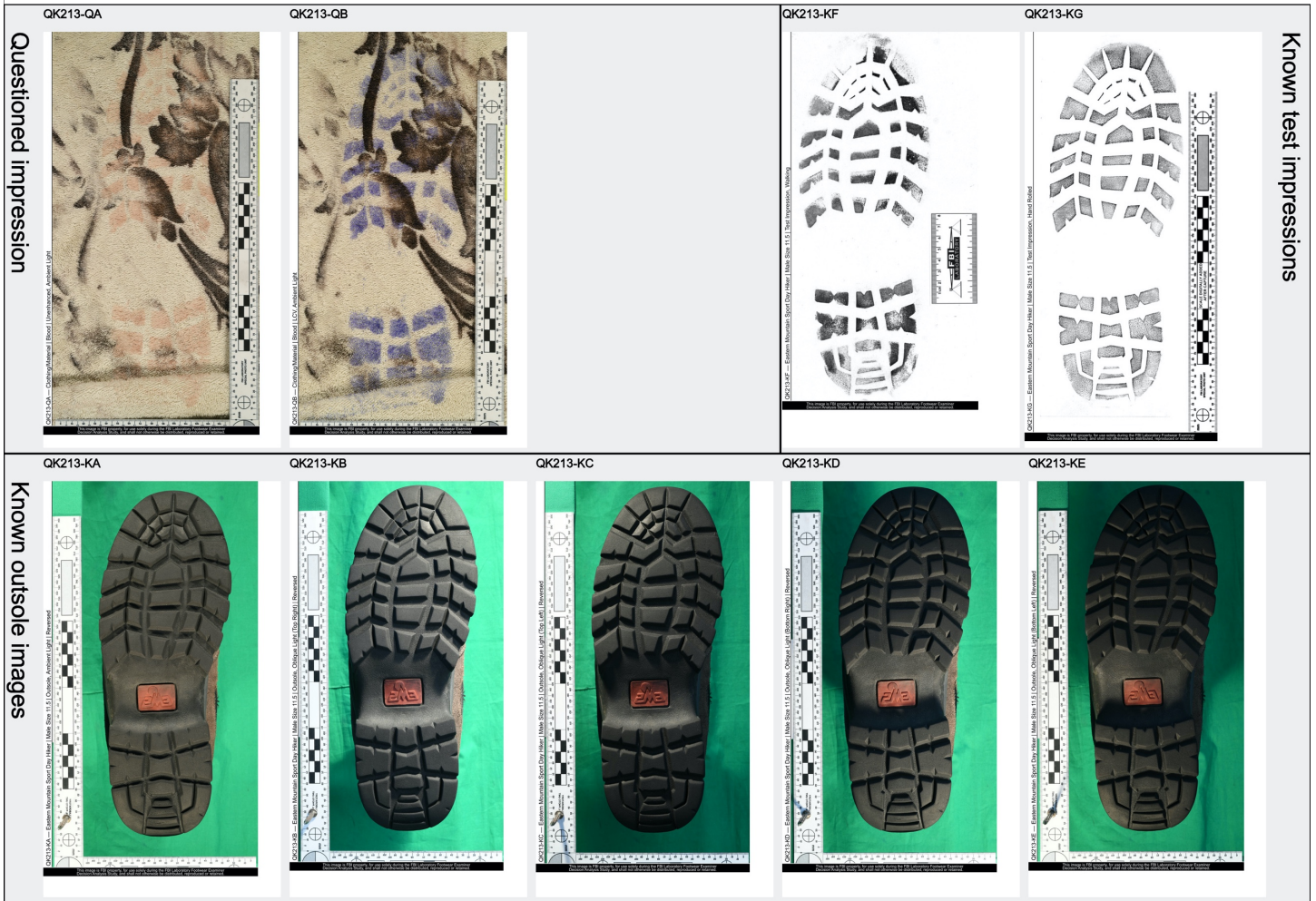
Figure 8. QK213: Mated QKset that resulted in 20 FNs. The questioned impression is synthetic blood on cloth (pre and post chemical enhancement). Conclusion rates for this QKset: 0 ID , 0 HighAssn , 0 Assn , 4 LimitedAssn , 0 Inc , 0 NotSuitable , 2 NonAssn , 20 Excl . Of the participants who concluded Excl , 2 reported that they observed differences in outsole design, and the remaining 18 reported differences in size between the questioned impression and known item of footwear. The majority of participants assessed the difficulty of this QKset as “easy,” which may be reflective of this perceived lack of class correspondence. See Appendix E3 for more detailed images.
