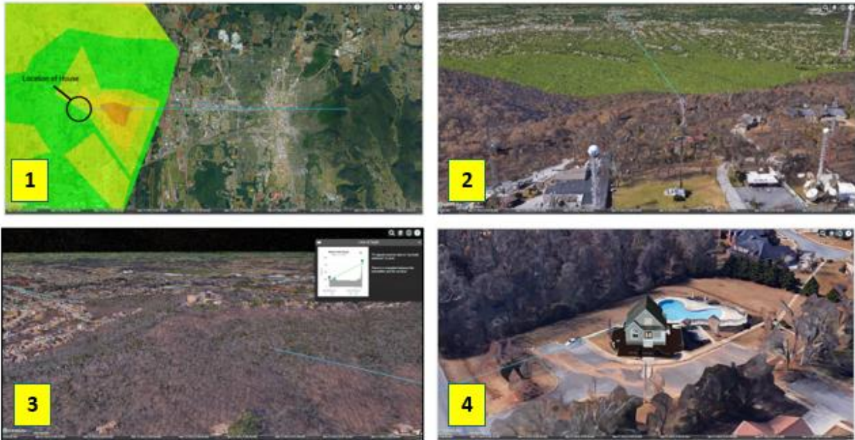
Figure 15 (1) RF Heat Map, (2) Transmitting Antenna Location, (3) Rainbow Mountain Blocking Line-of-Sight Between Transmitter and Receiver, (4) Receive Location
