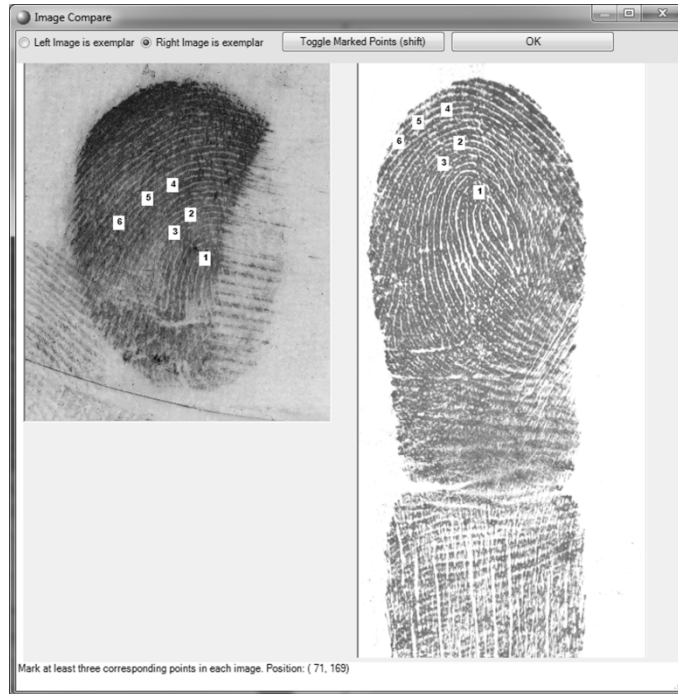
Figure 10: Example of the LQAS registration point user interface for marking corresponding points between and exemplar and latent print.
