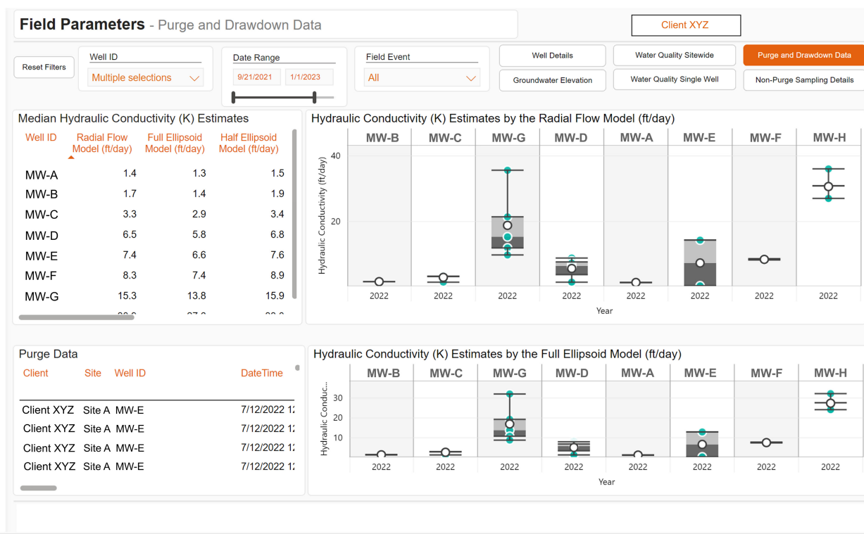
Figure 2. Low-Flow Drawdown Tool dashboard example showing hydraulic conductivity estimates for multiple wells over several sampling events.
